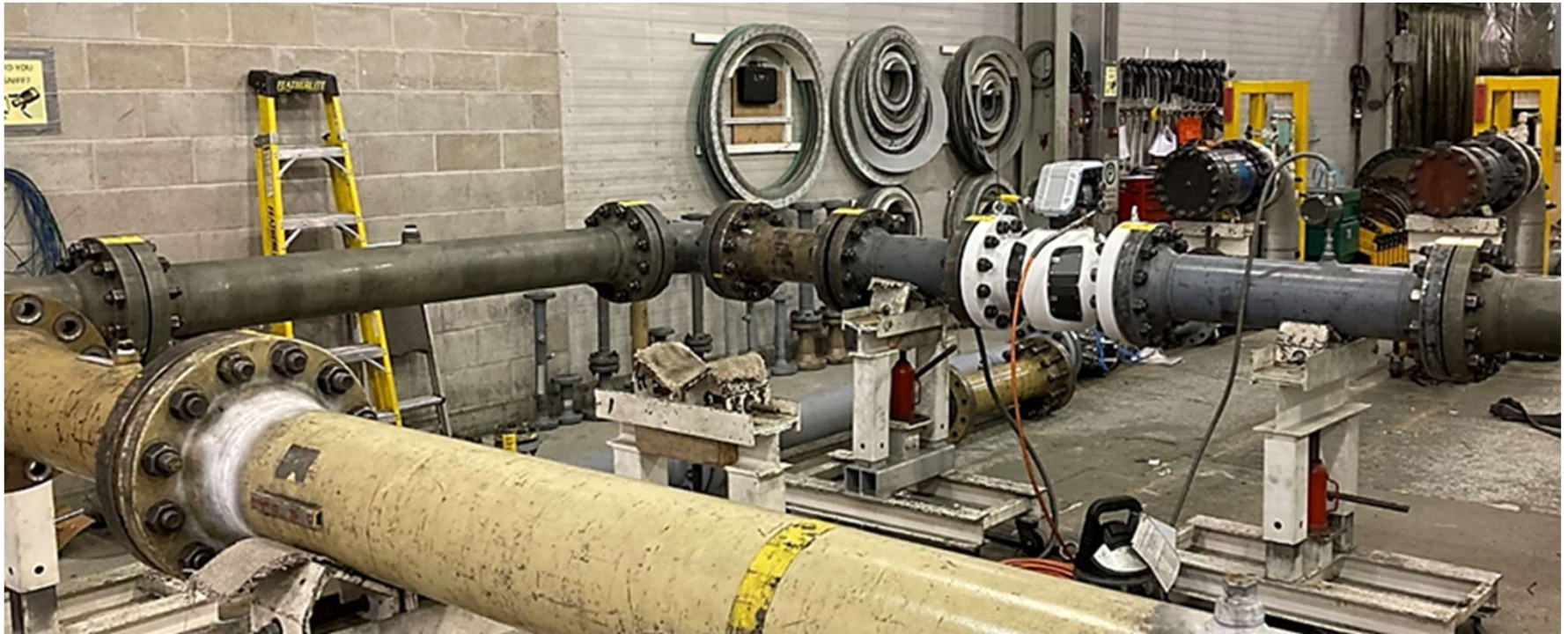
FLOWSIC600-XT Forte - Single Elbow Right Testing with 3D|CPA50E|3D
