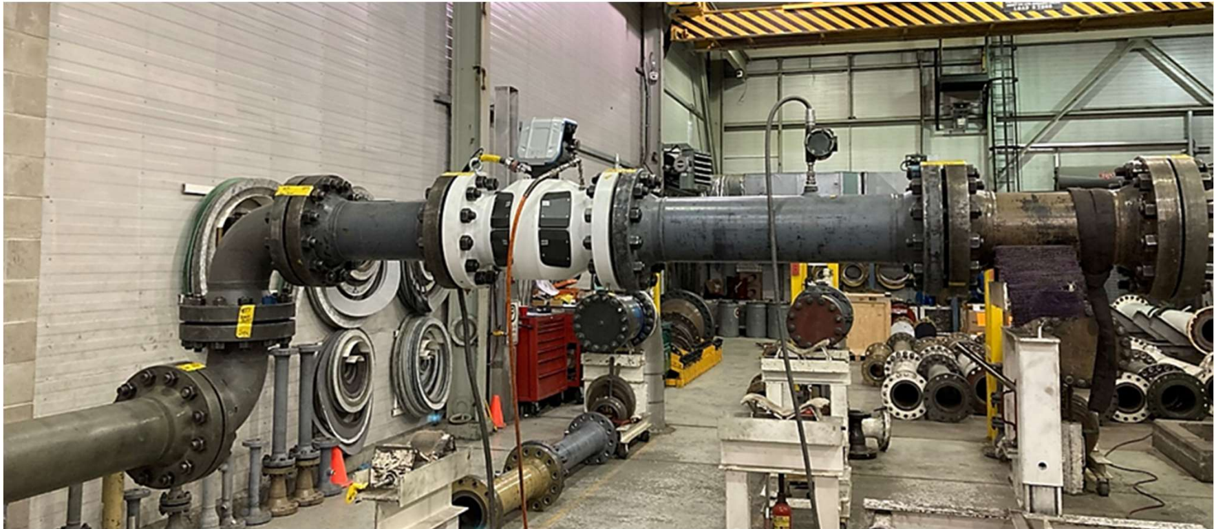
FLOWSIC600-XT Forte - Double Elbow Out of Plane Right Testing with 3D w/o FC
