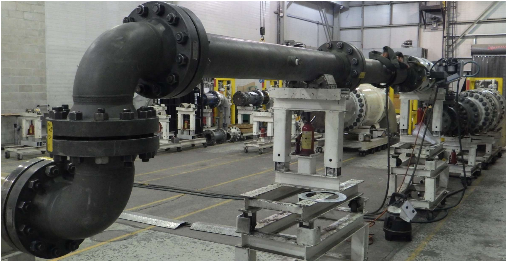
FLOWSIC600-XT 2plex - DEOOP LT - Double Elbow Out of Plane Left Turn 90 Degrees Testing with 10D|CPA50E|10D
