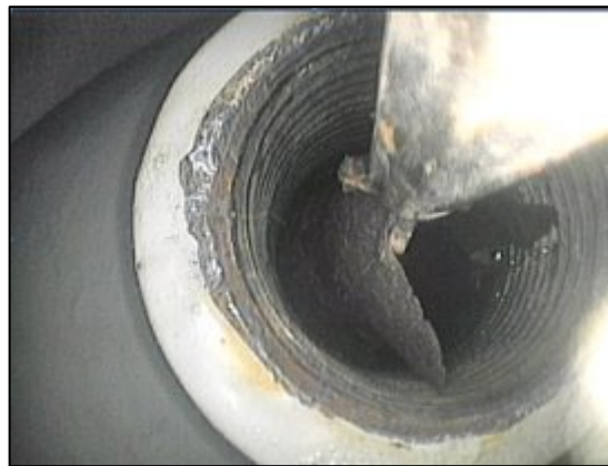
Removal of a piece of poly pig using a grabbing tool with borescope taped to the grabber
