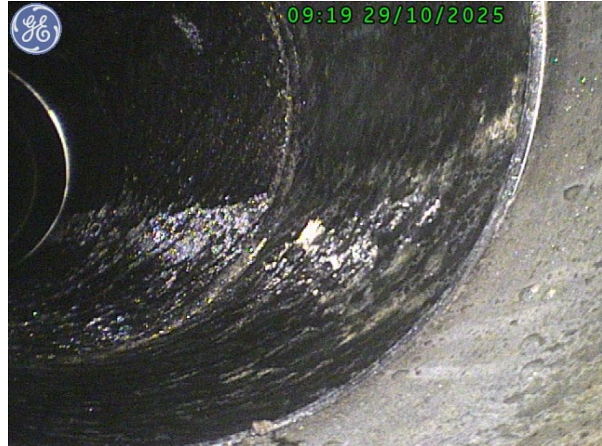
Spool #4 – Control spool uncoated. Typical low grade paint used on flanges/pipe prior to sale & fabrication. Notice the contamination congregating in the uncoated spool.
