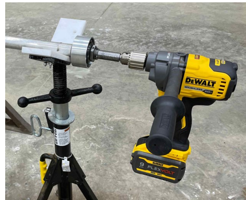
Dewalt 60V drywall mud mixing drill w/clutch sitting on Teflon blocked pipe stand.
