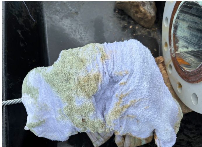
Ball hone wrapped in rag, post cleaning
