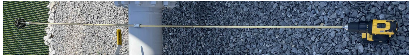
3" ball hone on chimney sweep rods
