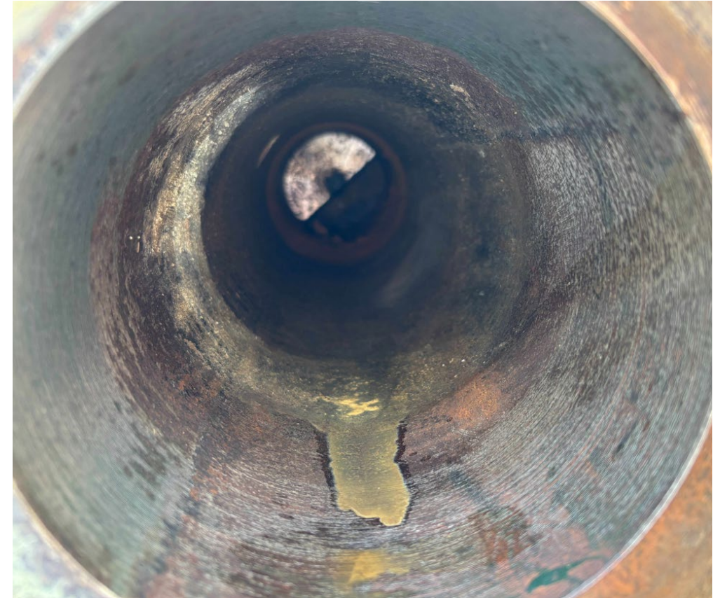
After final wiping by hand. Final condition. Some damage to coating by bare hone.
