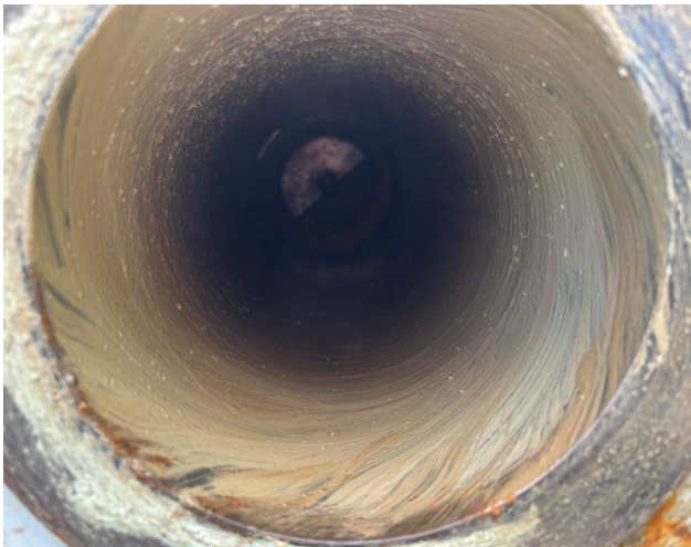
After 1 st ball hone cleaning. Hone covered by towel & degreaser used.
