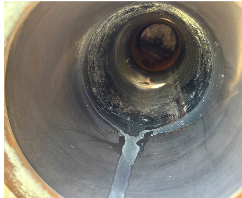
After final wiping by hand. Final condition. Minimal damage to coating by bare hone.
