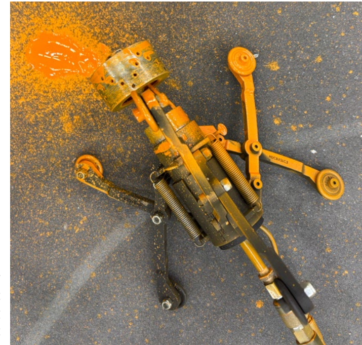
Rotary applicator just after applying a coat
