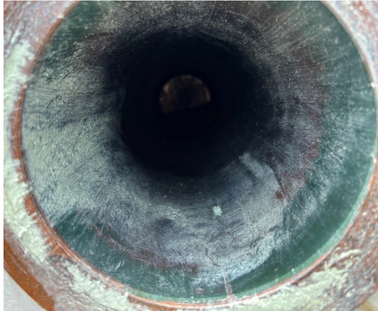
After 2 nd ball hone cleaning. Hone was bare & degreaser used.
