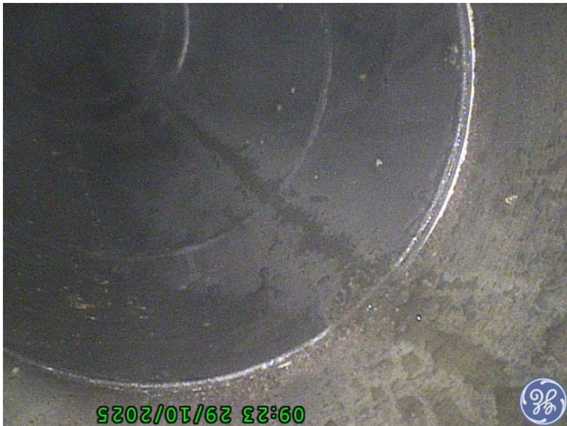
Spool #5 – Cerakote (black) and ambient cured. Notice more contamination lingering in the uncoated pipe adjacent to the coated spool.
