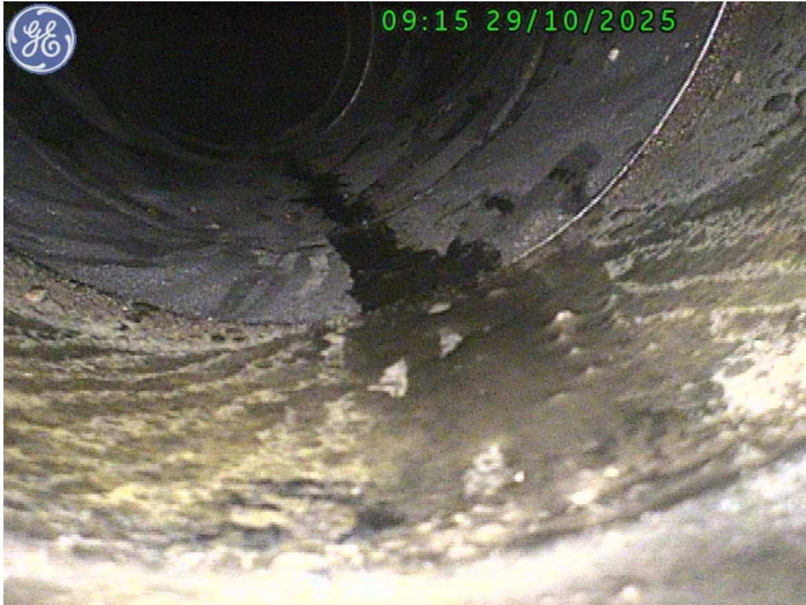
Spool #3 – Cerakote (black) and heat cured. Notice more contamination lingering in the uncoated pipe adjacent to the coated spool.
