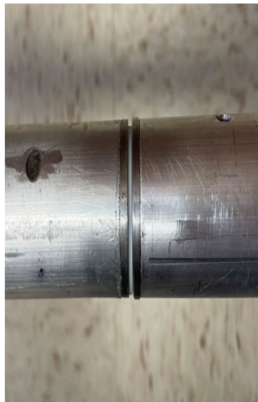
Tight rod to rod connection.
