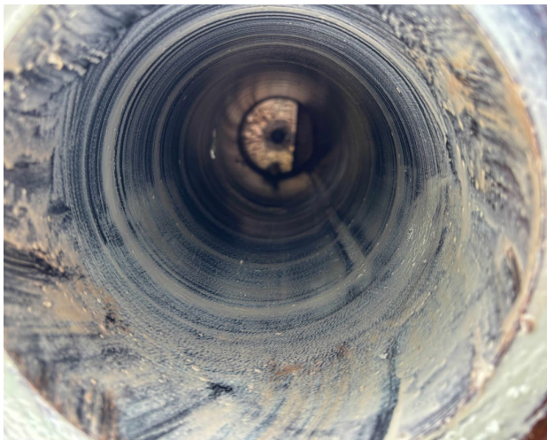
After 1 st ball hone cleaning. Hone covered by towel & degreaser used.
