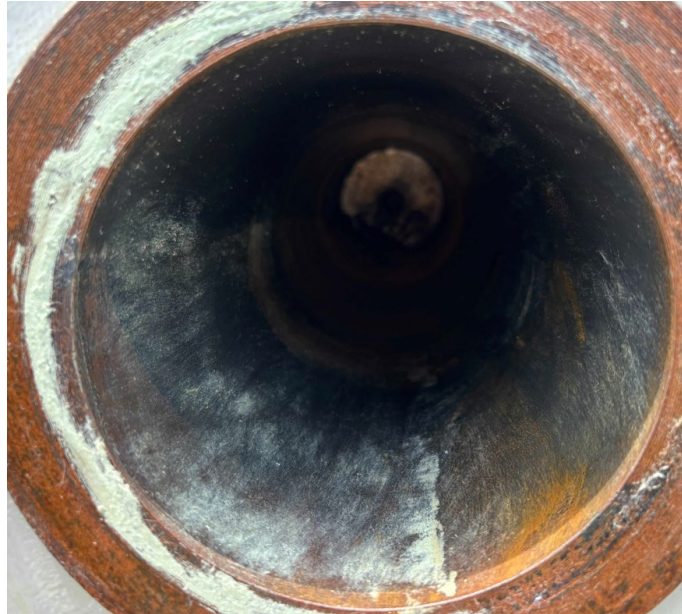
After 2 nd ball hone cleaning. Hone was bare & degreaser used.
