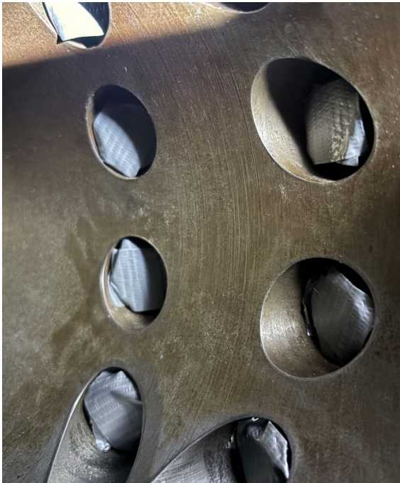
Transducer faces protected by duct tape (prior to blast)
