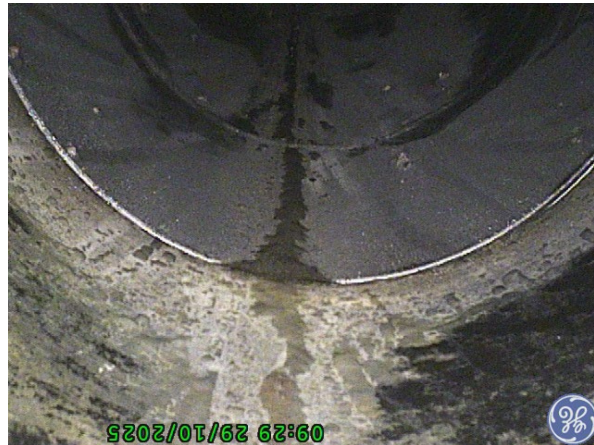
Spool #6 – Cerakote (black) and heat cured. Ball honed after coating to damage the coating.
