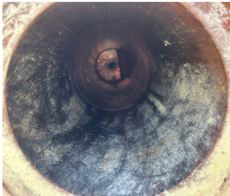
After 2 nd ball hone cleaning. Hone was bare & degreaser used.
