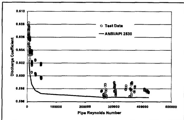
Figure 1. Orifice test data and ANSI/API 2530 discharge coefficients for 2" pipe Beta= 0.2413
