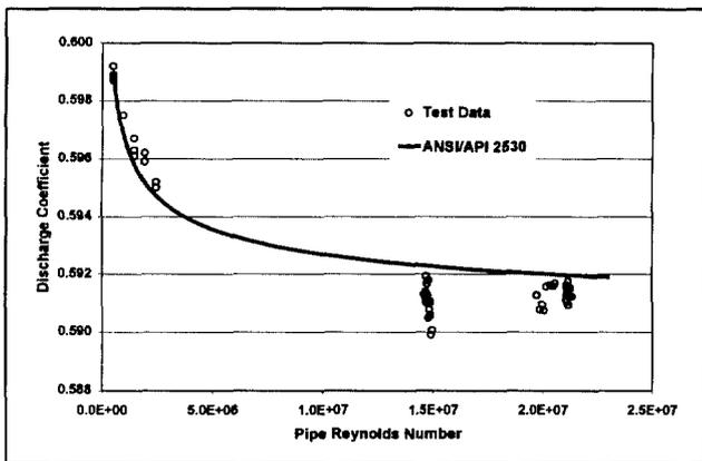
Figure 2. Orifice test data and ANSI/API 2530 discharge coefficient for 24" pipe Beta=0.7504
